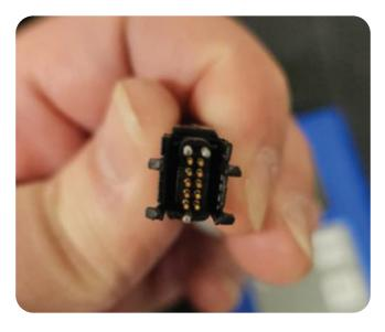
Secure the connection by pinching the plastic side clips of the connector until it snaps into place.
