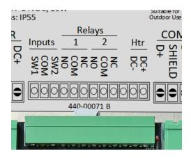
Relay 2's function is determined by the AP1's configuration setting. It can be set to function as an alarm output, slave to relay 1, slave to relay on with different on time, a heater controller (active when freezing temperatures occur) or activated only by the system controller.
